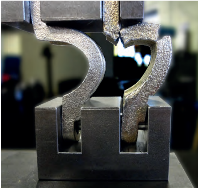
Fracture test - left: LÜDECKE hose clamp (no crack/ fracture), right: hose clamp from the Far East (complete fracture)
