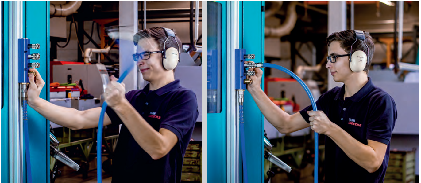
Whiplash-effect: high risk of injury when using compressed air - avoided through products from the LÜDECKE SafeConnect-Line .
