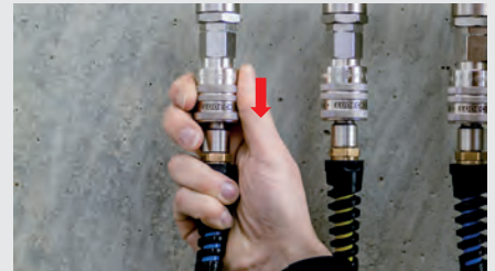
Disconnection - second step: Safe decoupling
