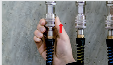
Disconnection - first step: Automatic venting
