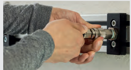
Two-hand operation: To disconnect, push the plug while pulling back the sleeve
